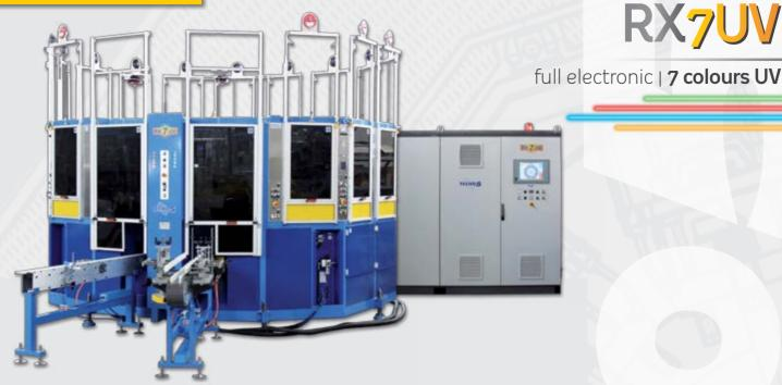
Automatic screen-printing machine servo-controlled suitable to print up to a 7 colours UV, designed for high printing precision on glass containers and tableware of different shape and dimensions.
